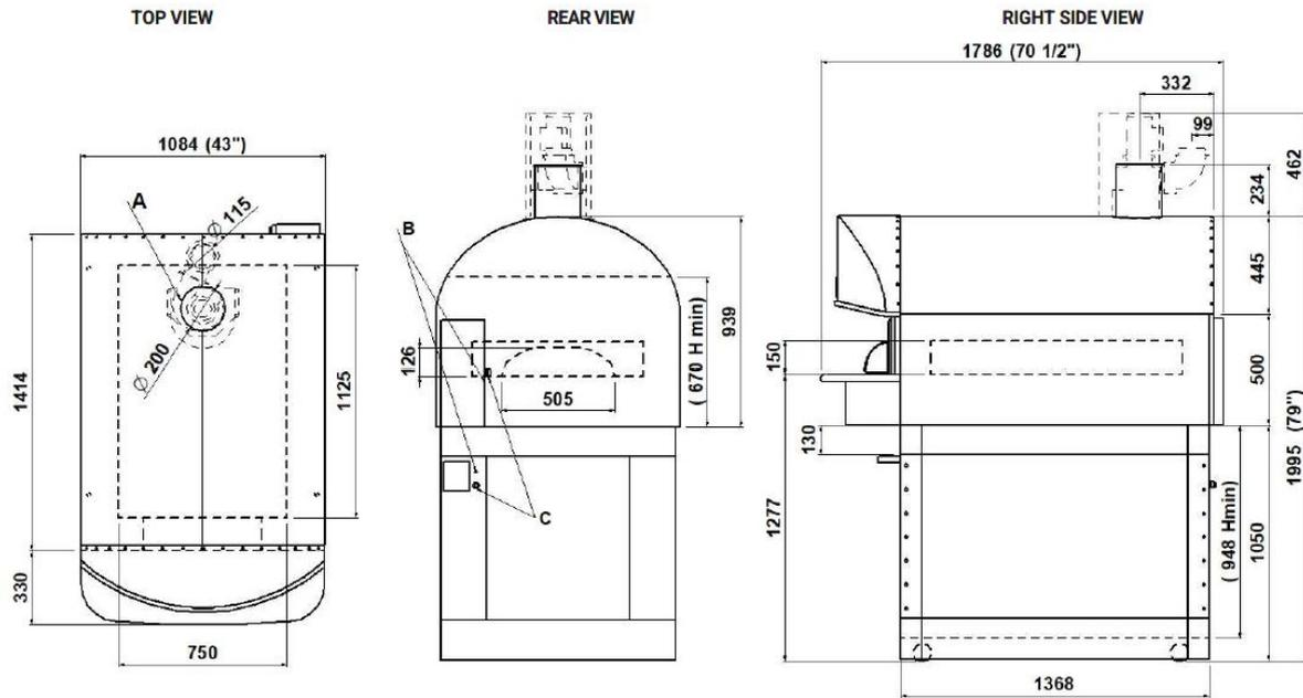
NOTE: The dimensions shown in these diagrams are in millimeters.
